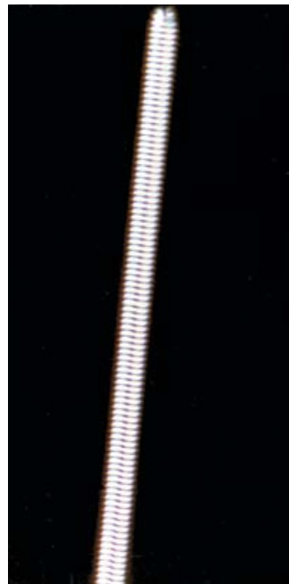
Figure 4. Photomicrograph of the characteristic growth of a spiral domain on slow cooling of the isotropic liquid of compound 15 , 146°C.
